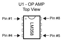
Note: Ensure the IC chip U1 (LM358) is wired correctly. The location of Pin #1 is shown above.
